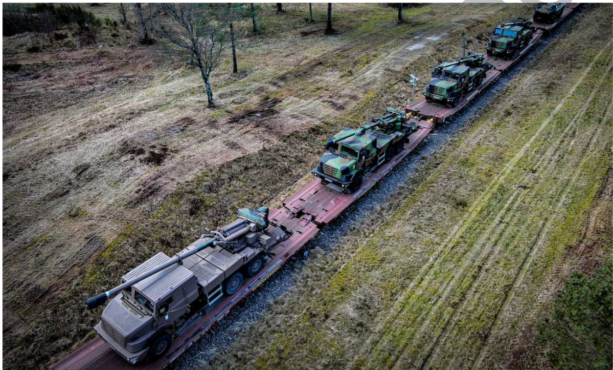
Figure 5: French Army SPH Caesar deployed by train for the Dynamic Front '23 exercise. Trains provide a fast way of transporting heavy howitzers. However, if necessary wheeled SPH can travel long distances by road thanks to their higher average speed, low fuel consumption and maintenance.
